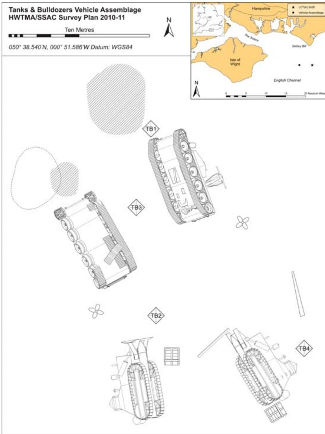
Figure 5.1. Location of monitoring points on the Tanks and Bulldozer vehicle assemblage.
