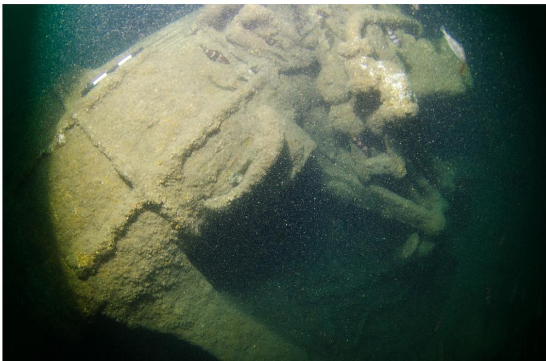
Figure 11: The triple expansion engine
