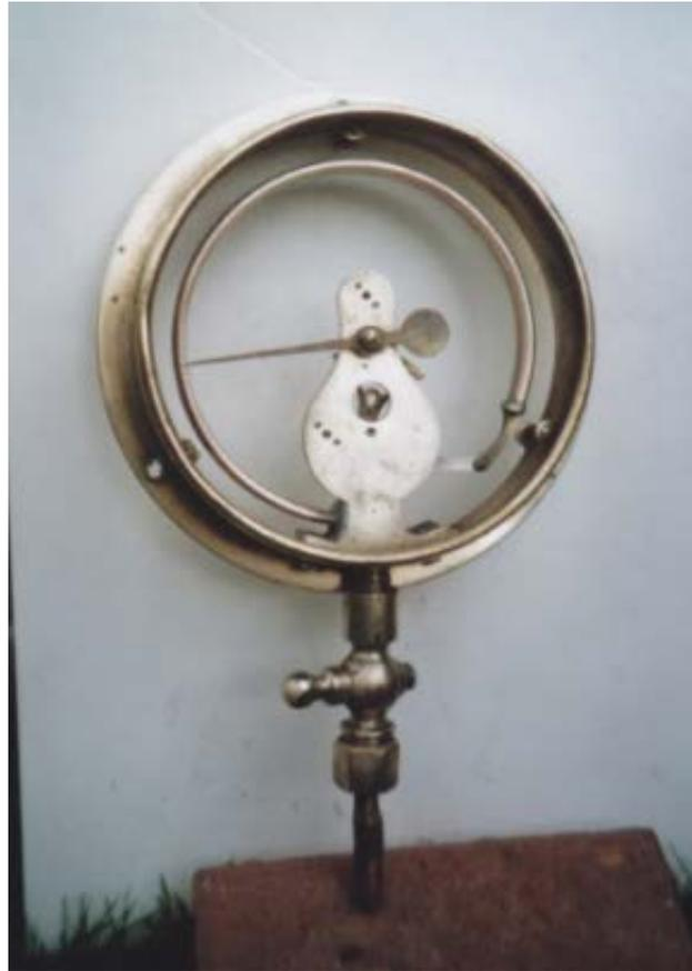
Figure 23: Steam pressure gauge from the *South Western*.
