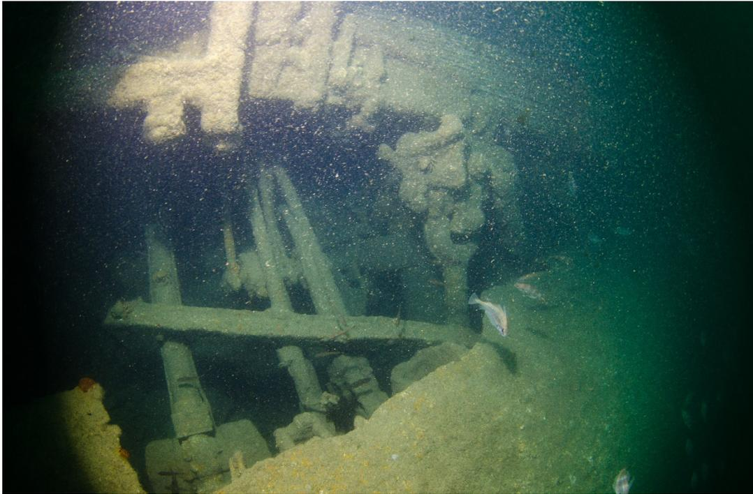
Figure 13: Part of the hull plating is resting on the engine
