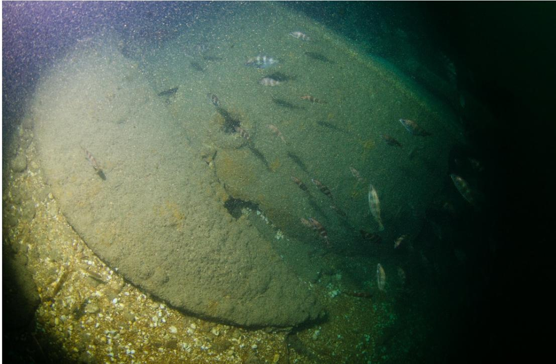
**Figure 18: Collapsed rudder**
