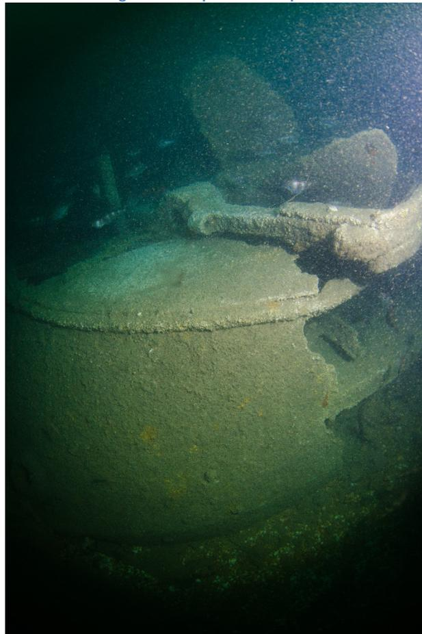
Figure 20: Propeller and rudder stock
