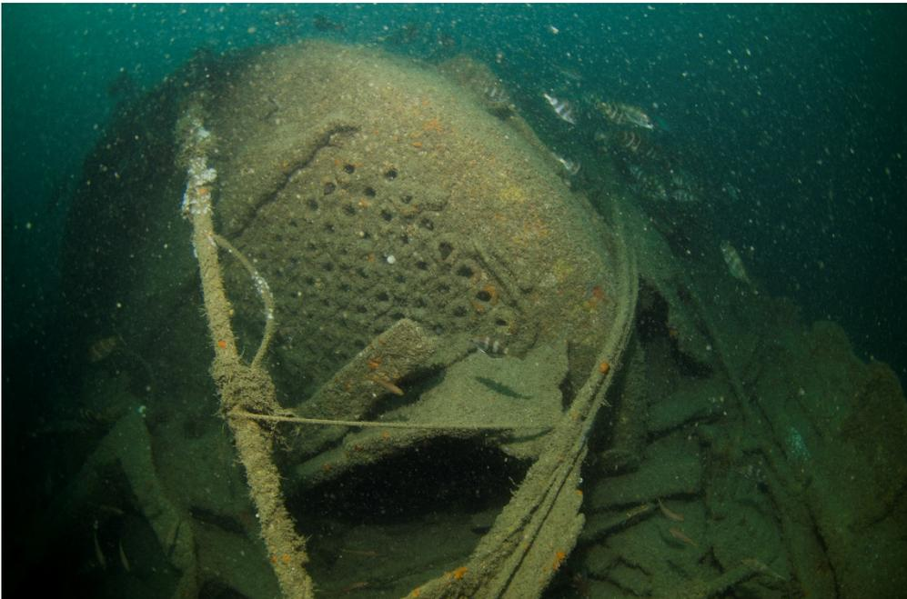
Figure 9: Boiler and steam pipes
