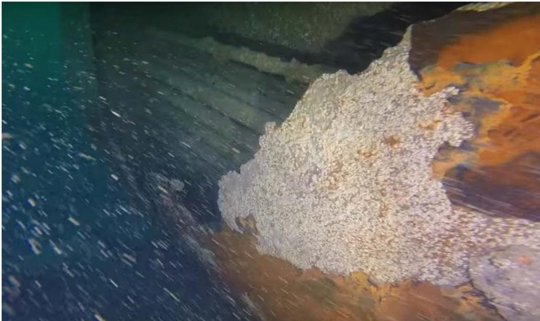
Figure 5: Boiler through which the fire tubes are visible (Courtesy of Dave Robbins)
