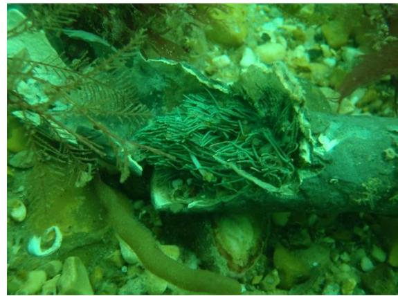
Figure 12: Twisted and broken lead piping (2011)
