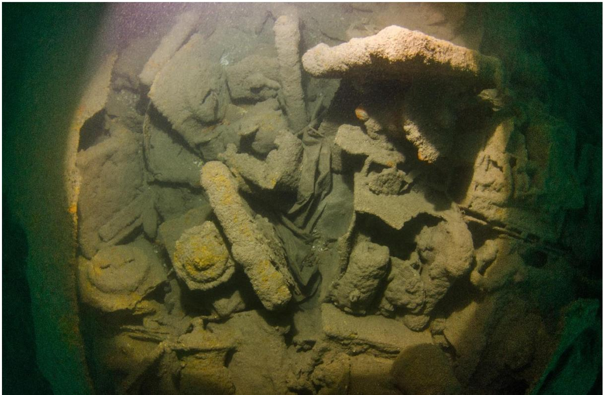
Figure 43: cargo packed into hold at stern, unidentified black sheeting (centre) can be seen amongst the cargo
