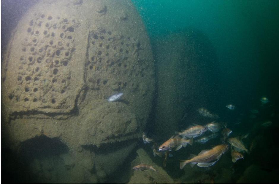
Figure 15: Forward end of boilers
