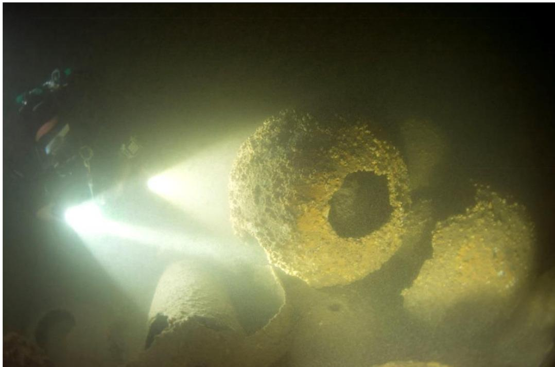
Figure 12: Mines photographed with powerful lights, corrosion of the munitions is evident ©Michael Pitts
