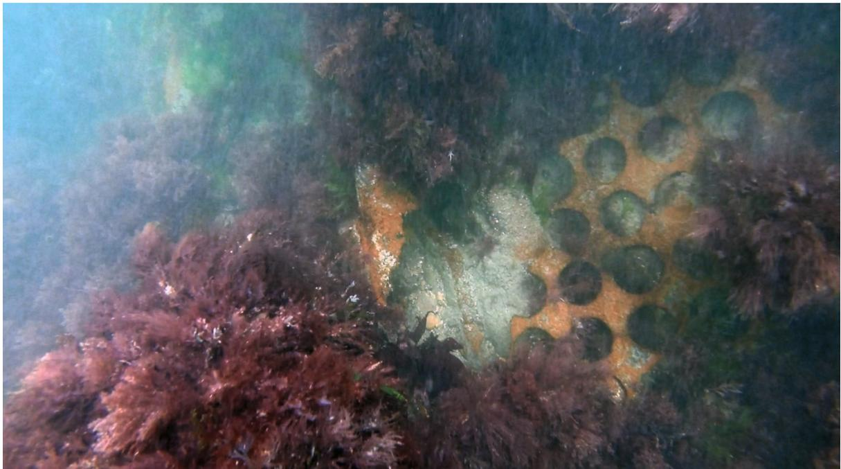
Figure 8: Part of the boiler, the holes once contained the fire tubes, the curve of the edge of the boiler can be seen to the left of the fire holes
